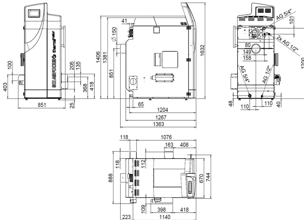
Caldaia a cippato thermi<sup>n</sup>ator II 49 e 60
