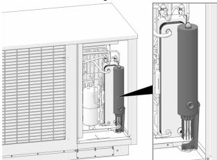
Abb. 2-7: Electric heating element mounted
