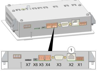
Abb. 2-45: Connections on the underside of the display
