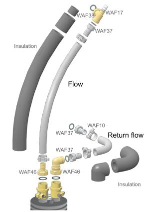
Abb. 2-29: Components of bottom connection set
