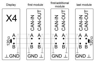
A 120 Ohm resistor is permanently installed in the display.
