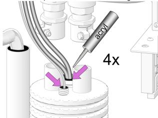
Abb. 2-39: Seal pipes
