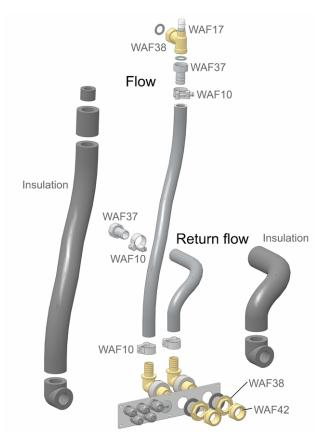
Abb. 2-33: Components of rear connection set
