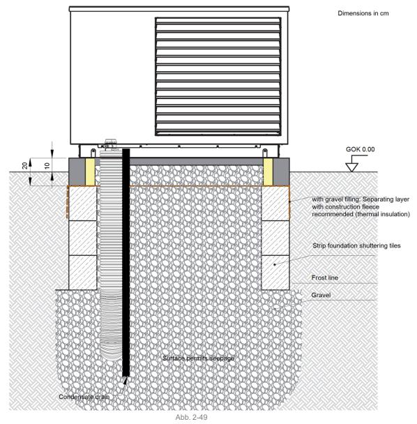
Detail B (illustration shows the heat pump pipe external diameter 40)
