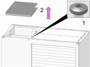
Abb. 2-36: Access to terminal area K 08, K 10
