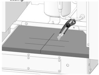
Abb. 2-27: Cut insulation mat
