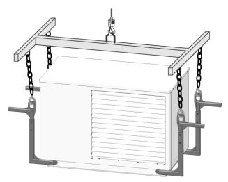
Abb. 2-13: Crane transport with lifting aid
