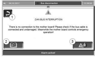
Fig. 2-60: Note window Fault
