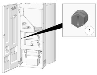
Fig. 2-1: Position of the overtemperature reset
