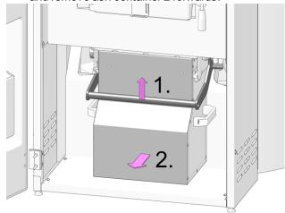
Fig. 2-52: Remove the ash container
