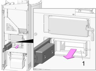
Fig. 2-55: Combustion chamber
