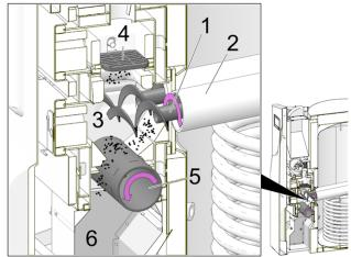
Fig. 2-50: Section through the burner
