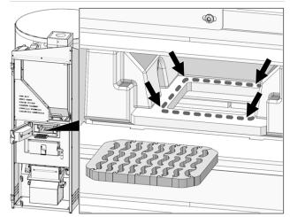
Fig. 2-54: Clean stainless steel combustion grate support surface
