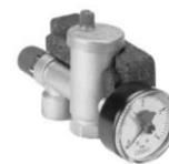
Install the BSG in the boiler supply line, at the highest point of the line, as close as possible to the boiler. Installation position: vertical, see illustration.
