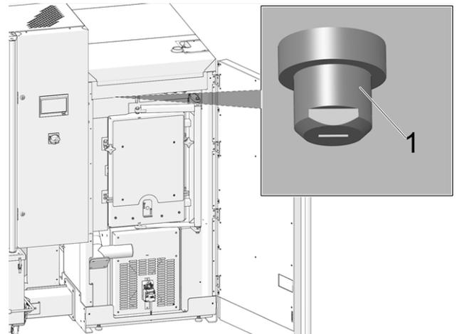
Abb. 2-3: Position of the overtemperature reset
