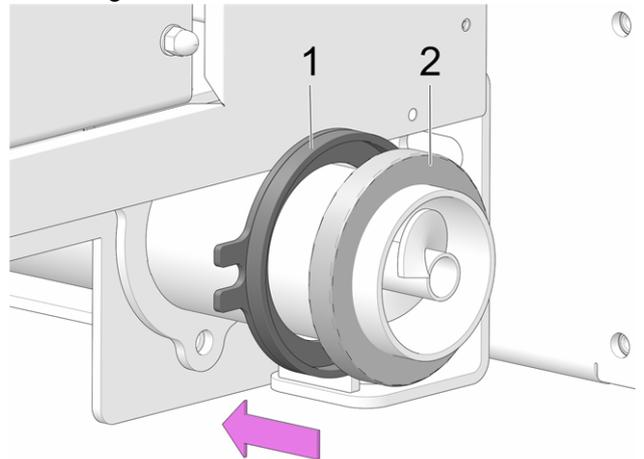
Abb. 2-24: Slide on sealing elements
