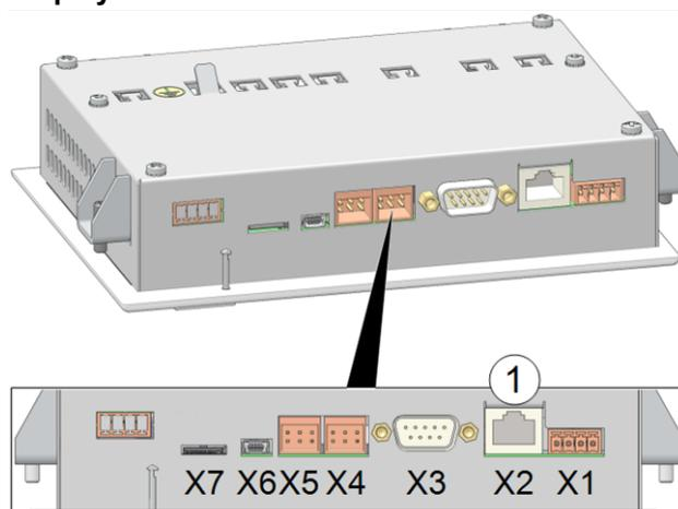
Abb. 2-63: Connections on the underside of the display
