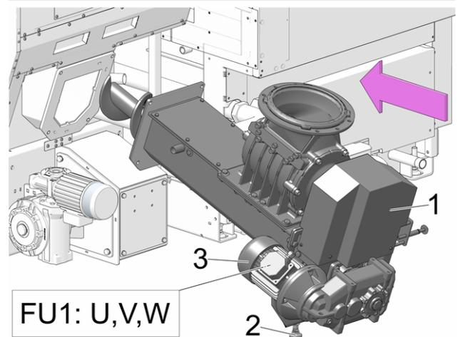
Abb. 2-34: Install the feeder unit
