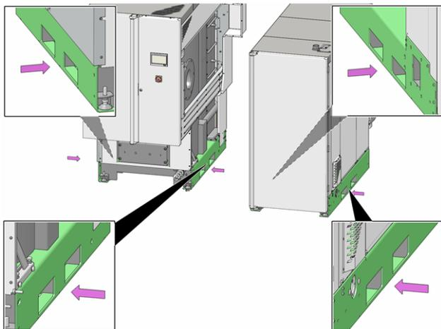
Abb. 2-14: Support points when taking load from side
