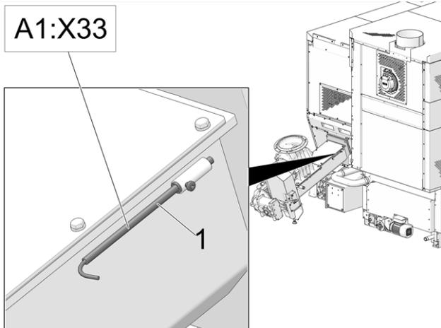
Abb. 2-35: Install the feeder sensor
