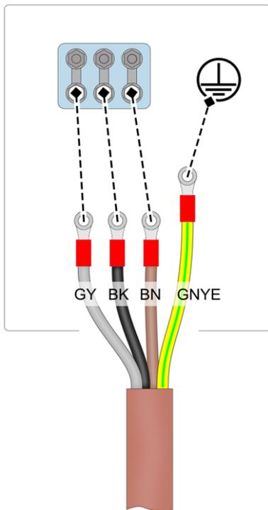
Abb. 2-36: Connect the cable in the motor terminal area
