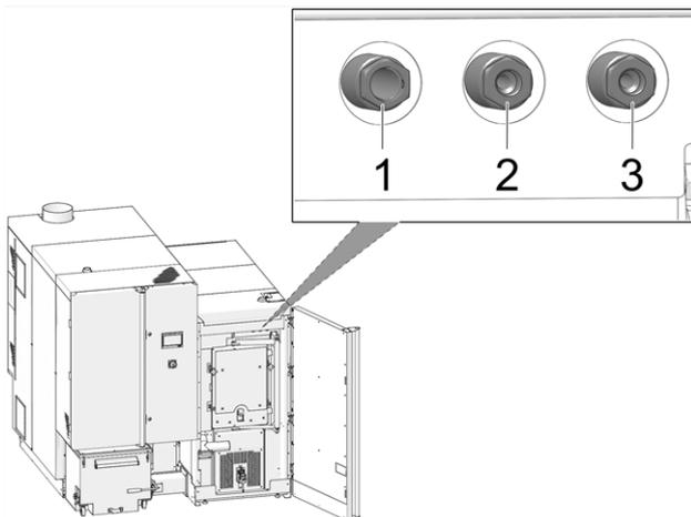
Abb. 2-47: Immersion sleeves on the burner
