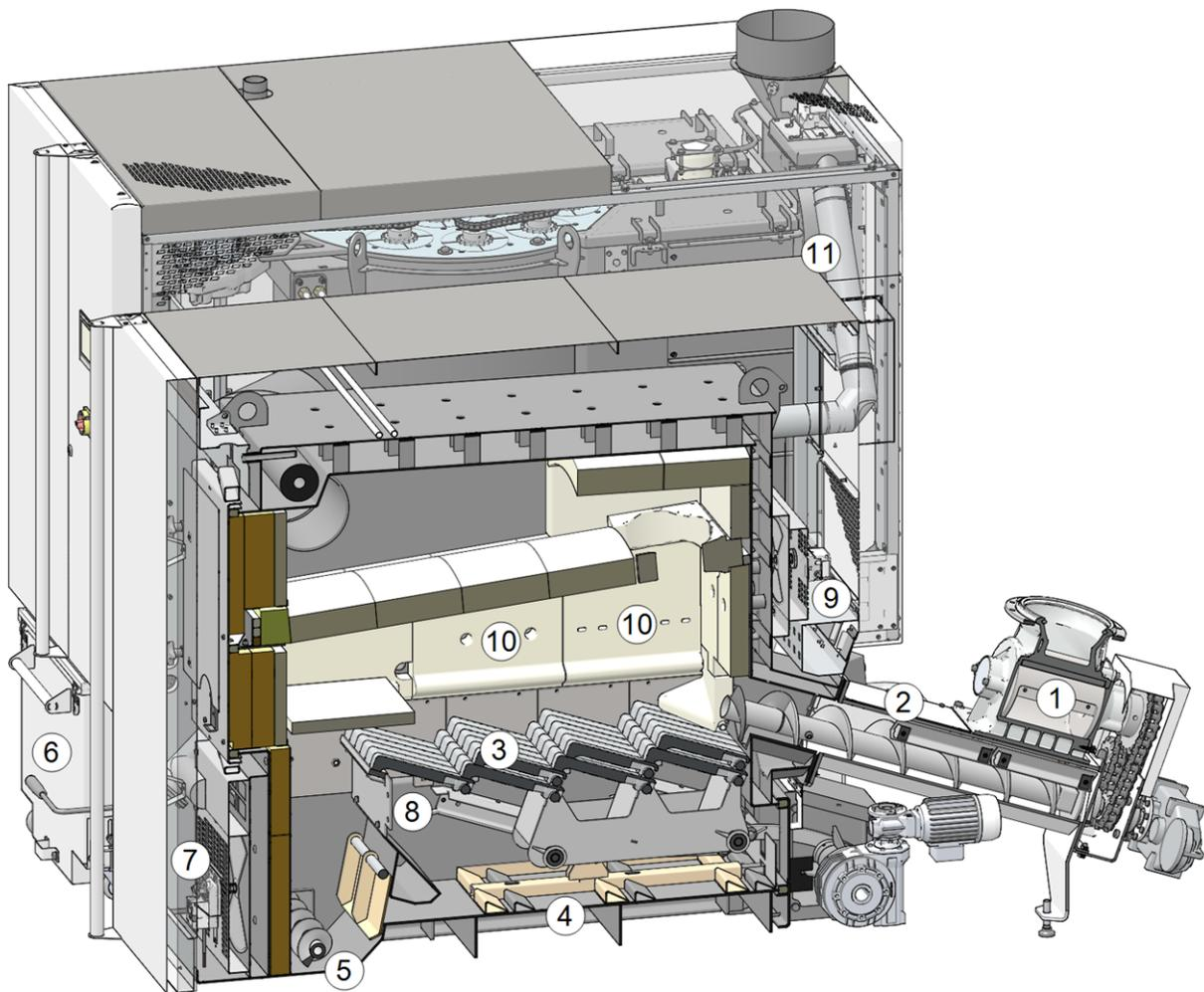
Abb. 2-12: Section through the burner
