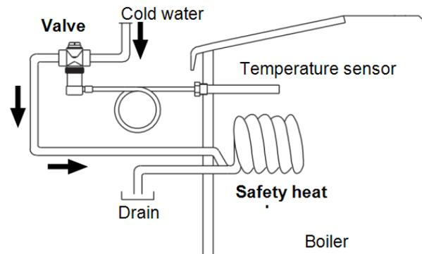
Abb. 2-40: Function of the thermal overload protection (schematic representation)
