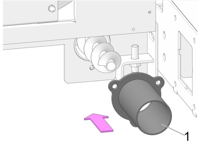
Abb. 2-23: Mount the auger channel
