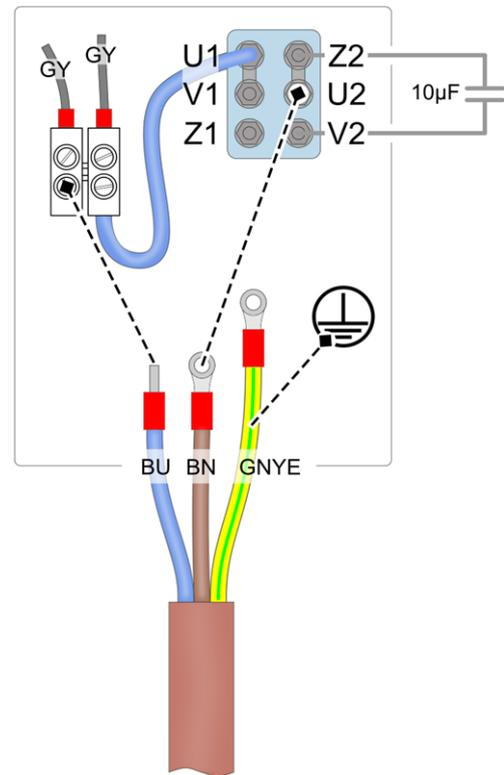
Abb. 2-33: Connect the cable in the motor terminal area
