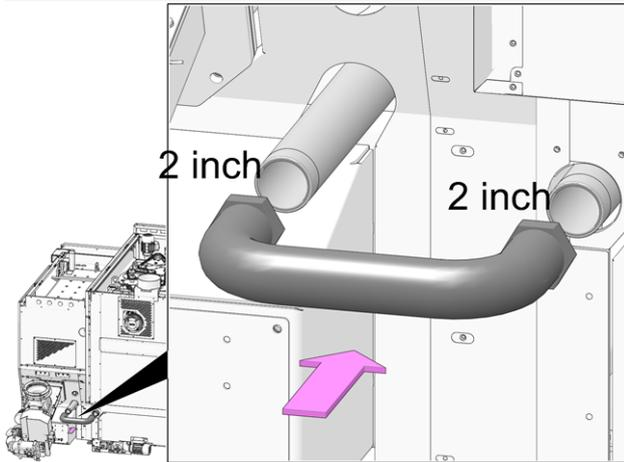
Abb. 2-31: Connect the water circuit
