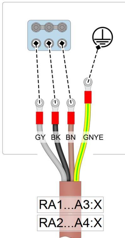
Abb. 2-60: Connect the cable in the motor terminal area
