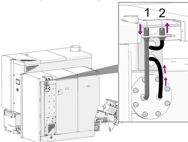
Abb. 2-38: Connect thermal overload protection
