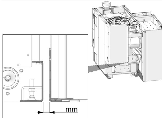
Abb. 2-20: Distance between the bottom plates
