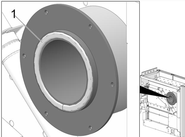
Abb. 2-18: Sealing cord in the flue gas pipe of the burner
