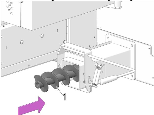
Abb. 2-28: Insert the auger
