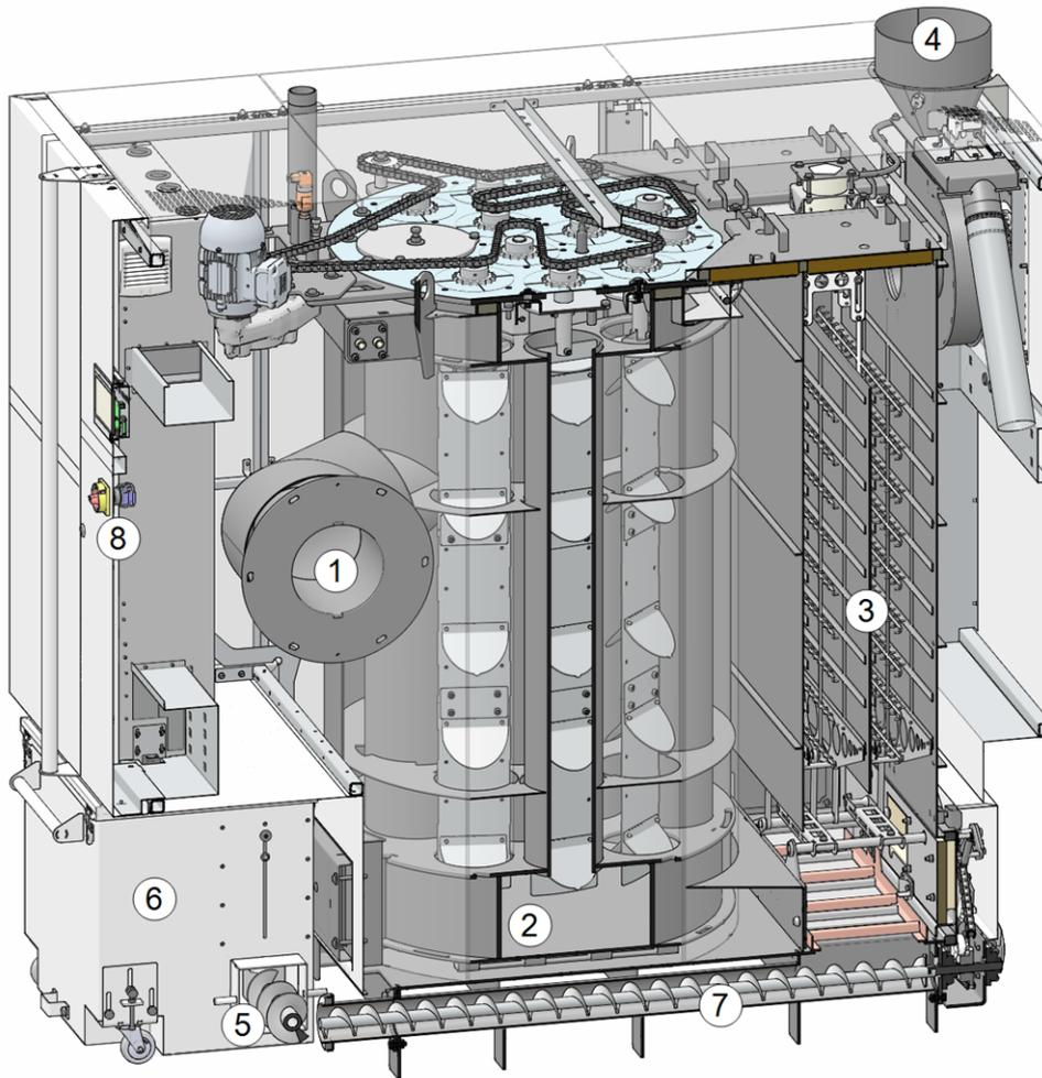
Abb. 2-13: Cross section through heat exchanger
