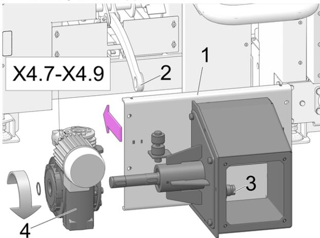
Abb. 2-32: Mount feeder grate drive
