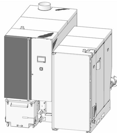
Abb. 2-51: Position of the control cabinet
