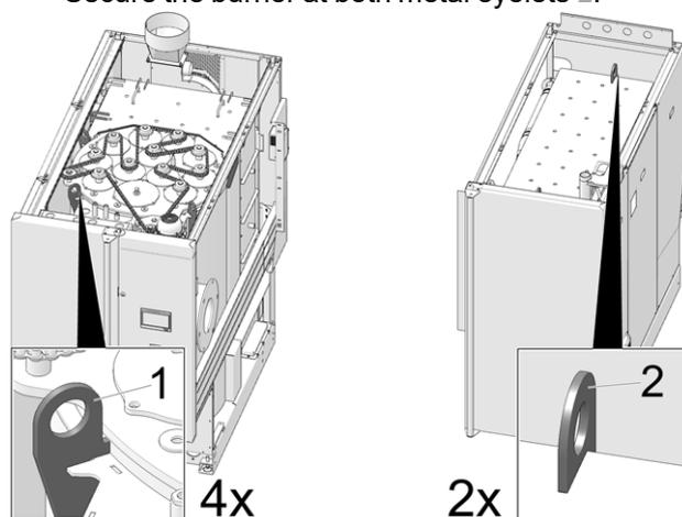
Abb. 2-16: Metal eyelets for crane transport
