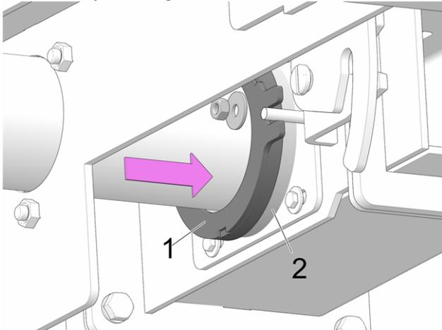
Abb. 2-27: Tighten sealing elements
