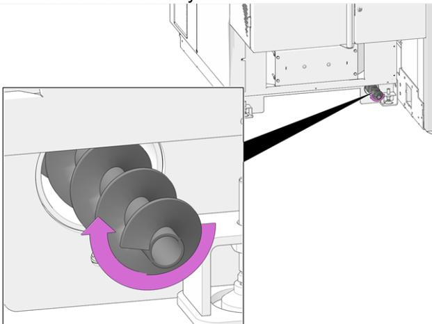
Abb. 2-22: Check auger drive
