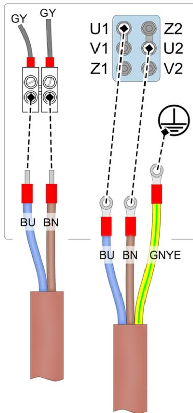
Abb. 2-71: Connect the cable in the motor terminal area
