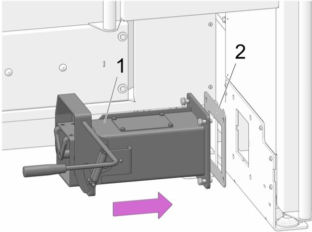
Abb. 2-26: Mount the auger channel
