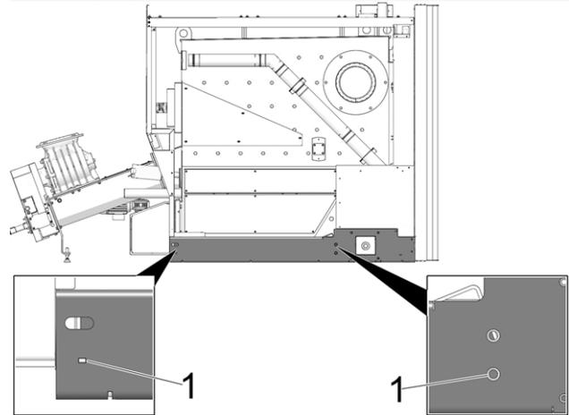
Abb. 2-19: Hole for screws
