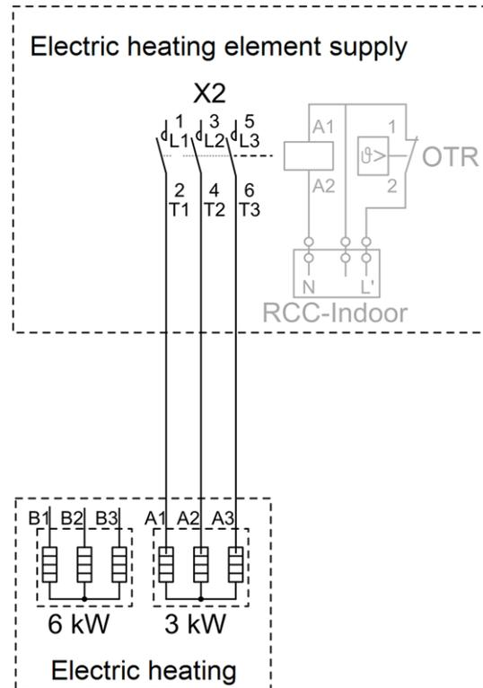
Power 6 kW: Connect wires B1, B2 and B3 to L1, L2 and L3.
