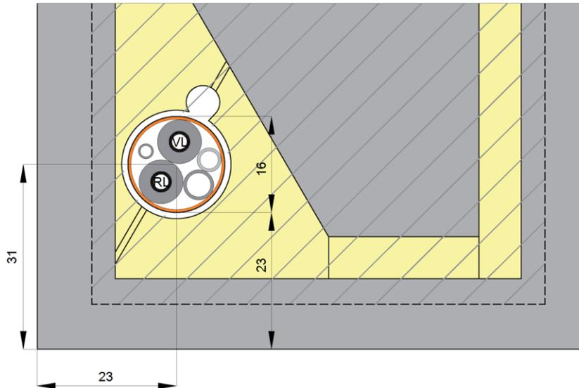
**Caution:** The position of the return pipe (RL) must be adhered to as precisely as possible.
