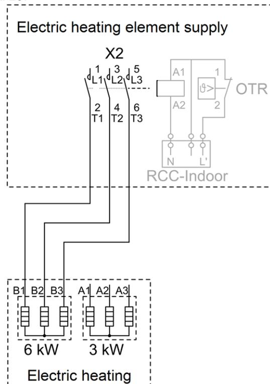
Power 9 kW: Connect wires A1 and B1 parallel to L1, A2 and B2 to L2, A3 and B3 to L3.
