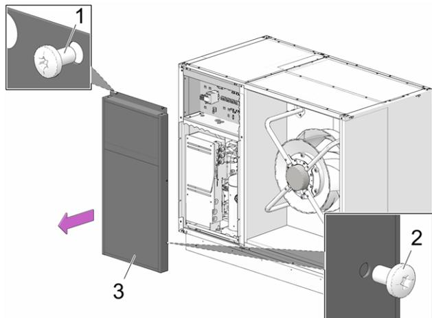
Abb. 2-38: Access to terminal area K 12, K 15
