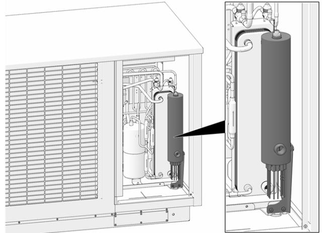
Abb. 2-7: Electric heating element mounted
