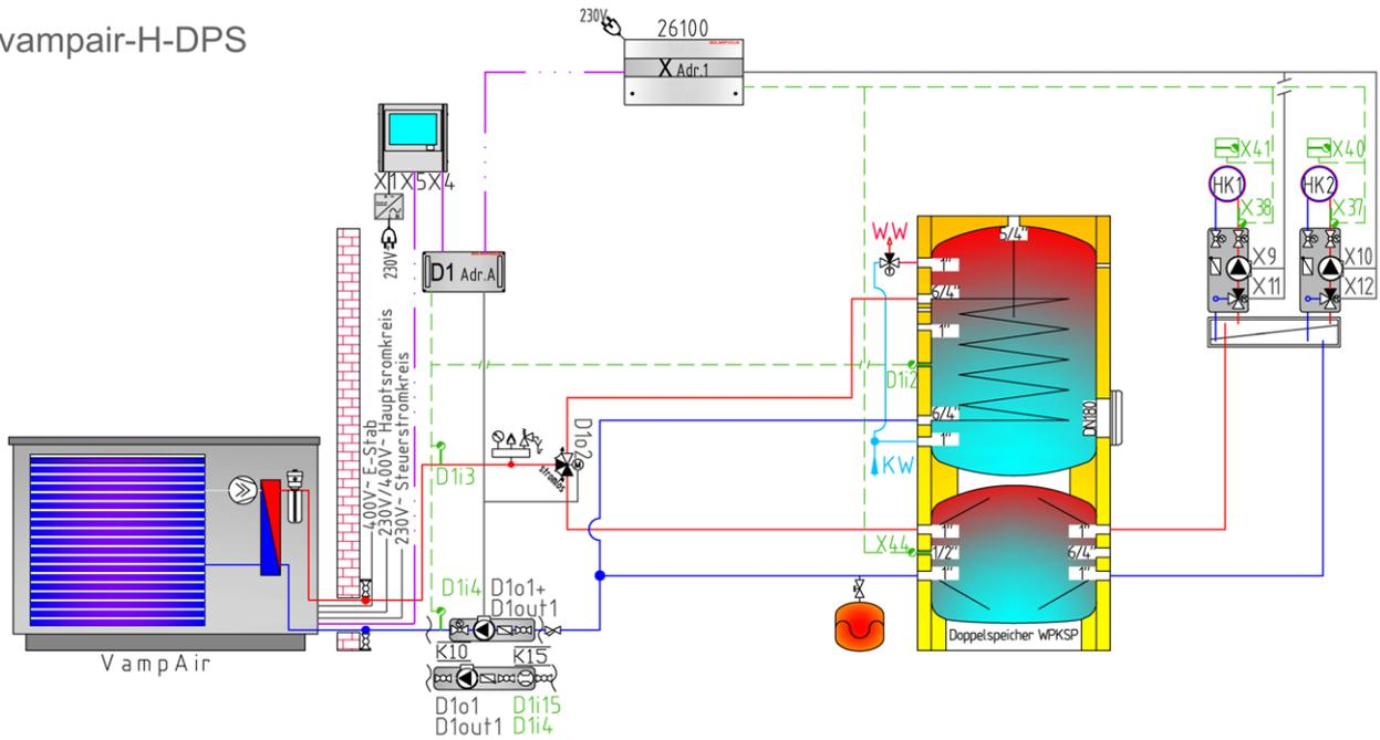
**vampair: for a mixed / unmixed heating circuit, with stratified buffer tank and fresh water module**
