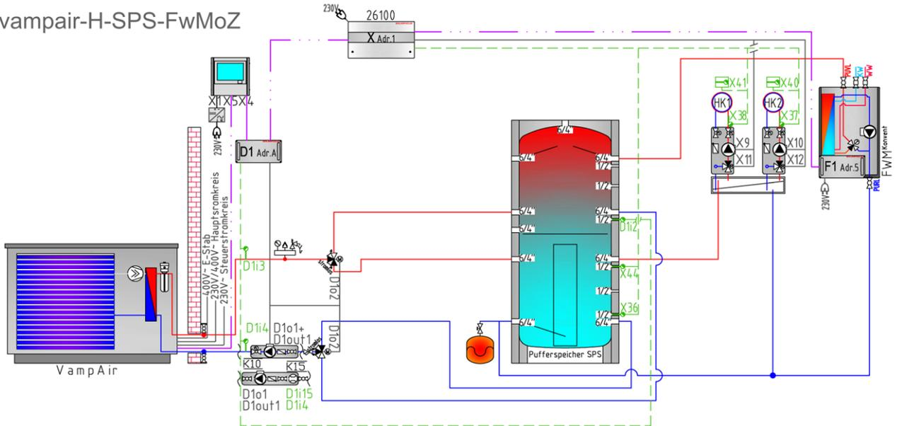
**vampair: for a mixed heating circuit, with stratified buffer tank incl. 2 solar coils and fresh water module**
