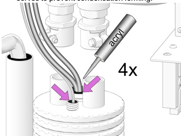
Abb. 2-39: Seal pipes
