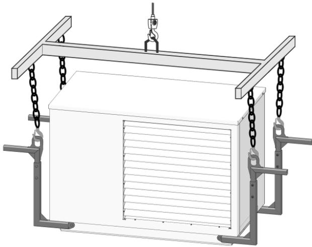
Abb. 2-13: Crane transport with lifting aid
