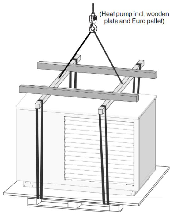
Abb. 2-12: Crane transport with Euro pallet (condition at delivery)
