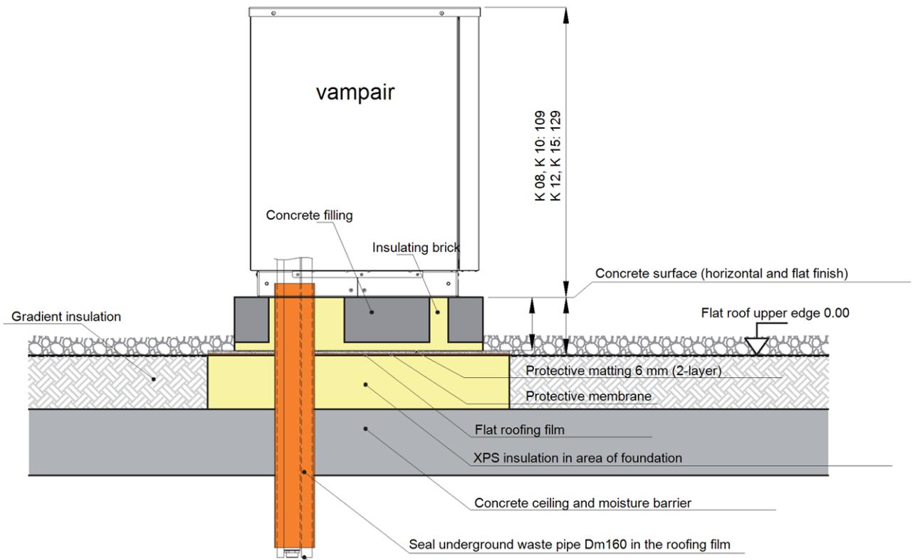
**Important information:** Seal cavity in underground waste pipe (KG) to make it diffusion-proof and airtight.
