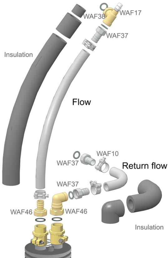
Abb. 2-29: Components of bottom connection set
