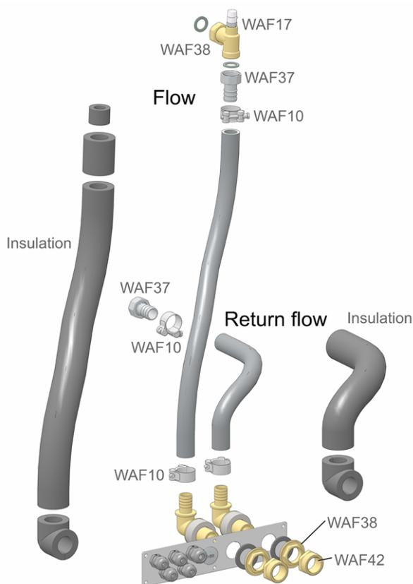
Abb. 2-33: Components of rear connection set
