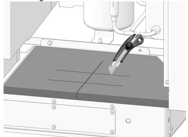
Abb. 2-27: Cut insulation mat
