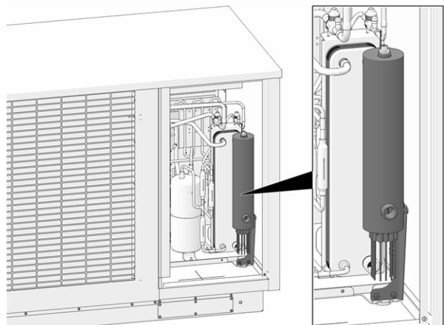
Abb. 2-6: Electric heating element mounted
