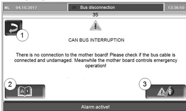
Fig. 2-60: Note window Fault
