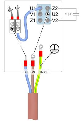
Abb. 2-33: Connect the cable in the motor terminal area
