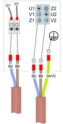
Abb. 2-71: Connect the cable in the motor terminal area
