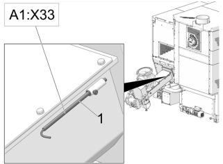
Abb. 2-35: Install the feeder sensor
