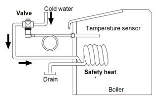
Abb. 2-40: Function of the thermal overload protection (schematic representation)
