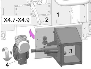
Abb. 2-32: Mount feeder grate drive
