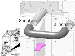
Abb. 2-31: Connect the water circuit
