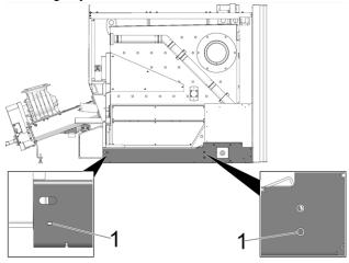
Abb. 2-19: Hole for screws
