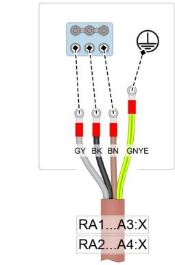
Abb. 2-60: Connect the cable in the motor terminal area
