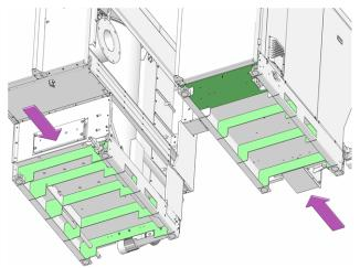
Abb. 2-15: Support when taking load from front, rear
