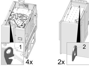
Abb. 2-16: Metal eyelets for crane transport
