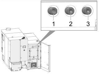
Abb. 2-47: Immersion sleeves on the burner
