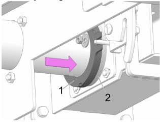
Abb. 2-27: Tighten sealing elements
