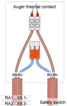
Abb. 2-62: Connect the safety switch in the motor terminal area
