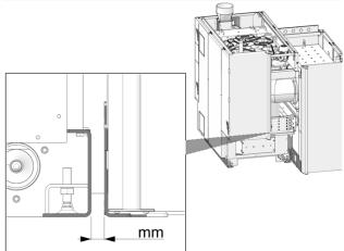
Abb. 2-20: Distance between the bottom plates
