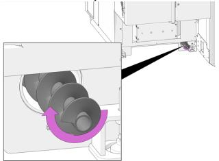
Abb. 2-22: Check auger drive
