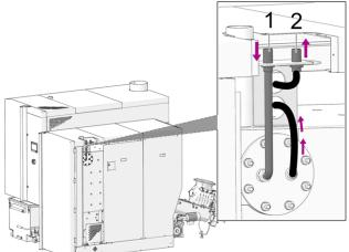
Abb. 2-38: Connect thermal overload protection
