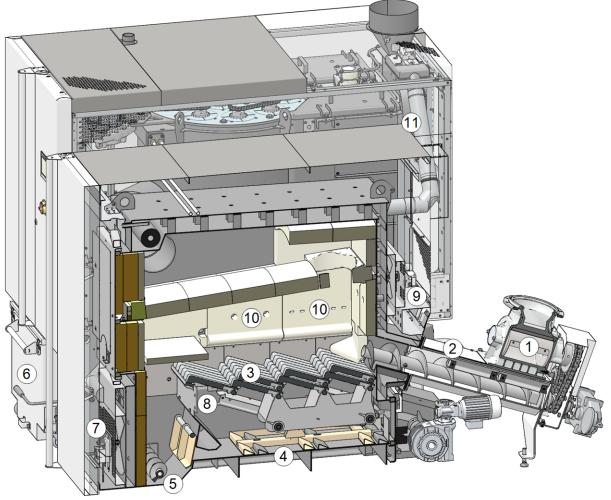
Abb. 2-12: Section through the burner
