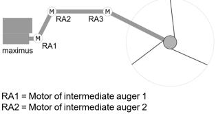
RA3 = Motor of direct extraction auger (see separate manual DR-0214)
