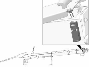
Opening the channel cover interrupts the power supply to the auger motor.
