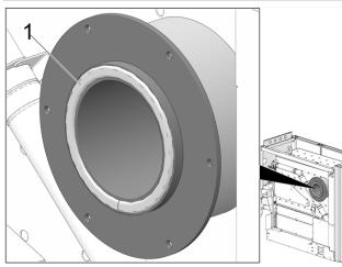
Abb. 2-18: Sealing cord in the flue gas pipe of the burner
