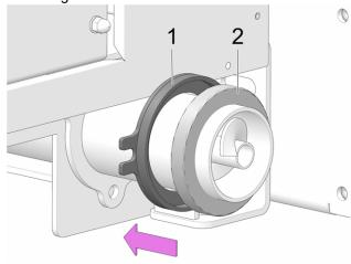
Abb. 2-24: Slide on sealing elements
