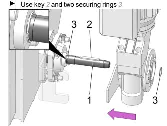
Abb. 2-29: Drive on right side of burner
