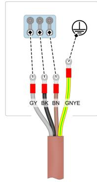
Abb. 2-36: Connect the cable in the motor terminal area
