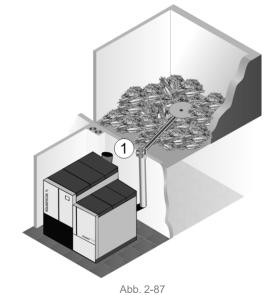
1 Direct extraction auger motor (=*direct extraction motor 1*), connection **A3:X2**
