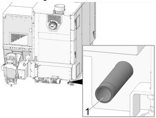
Abb. 2-49: Draining on the back of the heat exchanger
