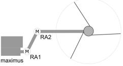
RA1 = Motor of intermediate auger RA2 = Motor of direct extraction auger
