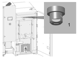
Abb. 2-3: Position of the overtemperature reset
