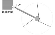
RA1 = Motor of direct extraction auger
