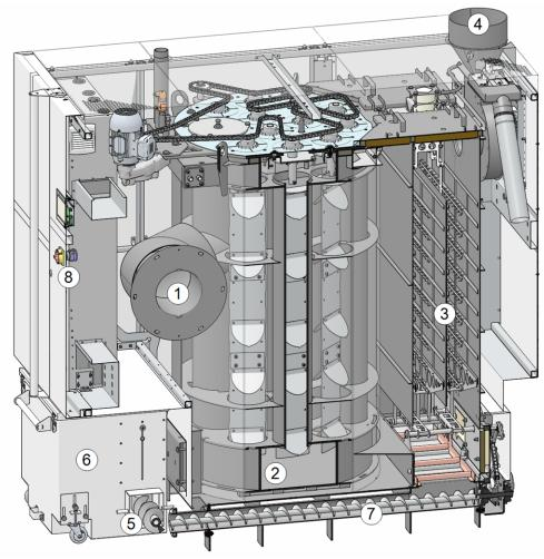
Abb. 2-13: Cross section through heat exchanger
