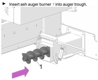
Abb. 2-28: Insert the auger
